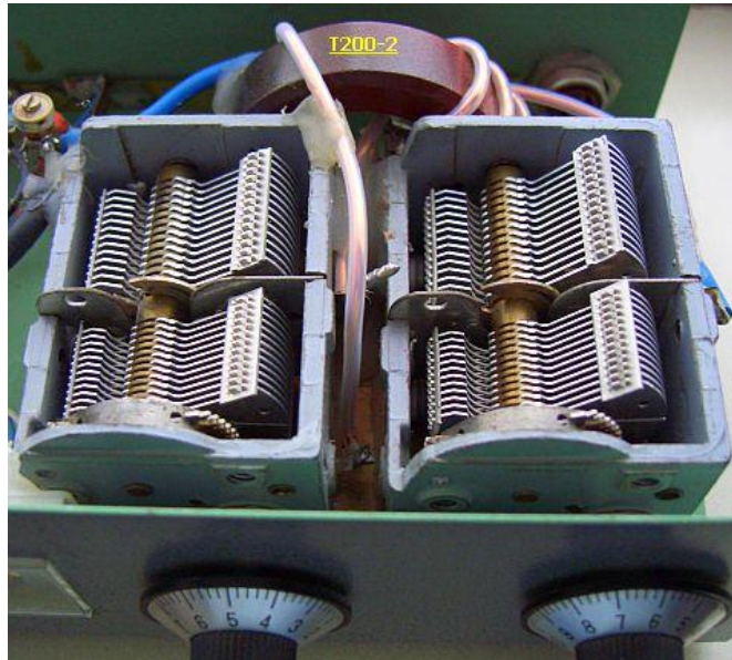
Home-made ATU (width), 17.5 6 12 cm with a T200-2 toroid:
