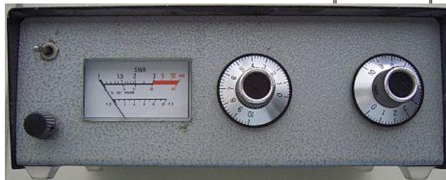
Home-made ATU (width), 17.5 6 12 cm with a T200-2 toroid:
