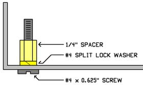
Before the PA mosfets can be mounted, the bottom piece of the case must be prepared by inserting the four board mounting screws and threaded spacers. Insert a # 4 x 0.625" screw in the corner holes on the bottom case piece, add a split lock washer, then secure with the 1/4" long threaded hex spacer. Do this in each of the four corners.
