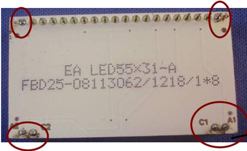
The back lighting module needs to be soldered to the bottom of the display. Only the two corner pins on the 20 pin row need to be soldered to support that end. Soldering more than these corner pins would make it very difficult to replace the back lighting module, should that ever be needed.
