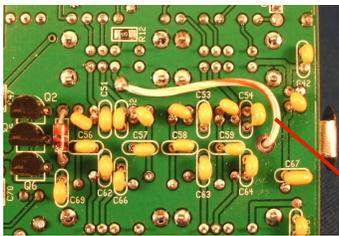
A wire used to connect the antenna connector to the board is now added.
