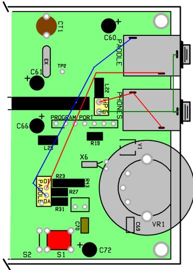
Use the # 26 Teflon wire (white/blue stripe) for these connections. A separate ground wire is not used for the paddle jack and gets its ground using a wire jumper over from the headphone jack. Route the wires as shown in the photo.
