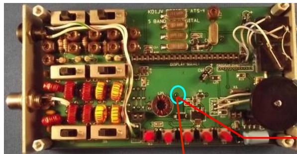
DDS test point. Attach temp wire here and run to front of case
