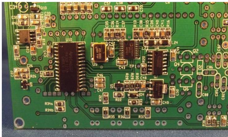
Since the number one reason a kit does not work the very first time power is applied is due to soldering issues, it is well worth it to spend time now carefully inspecting your soldering. Finding and correcting these problems now will save you much time and frustration trying to find them later. Use a magnifying glass to inspect the connections to each part and IC lead. There are several things to look for.
