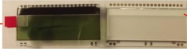
Remove film from top of back lighting module before soldering to bottom of display module.
